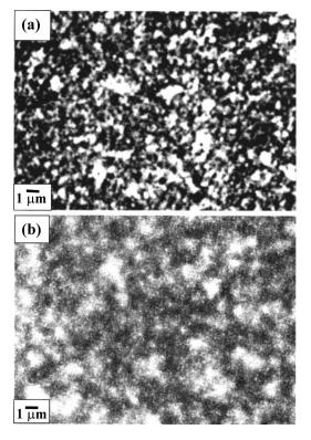
FIG. 3. (a) Typical CL image before thermal annealing; (b) typical CL image after thermal annealing.
