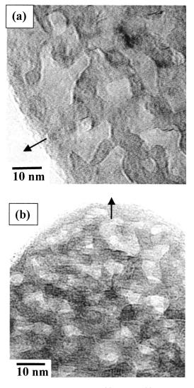
FIG. 5. Typical HRTEM images before (a) and after (b) thermal annealing. Arrows show crystal growth directions.
